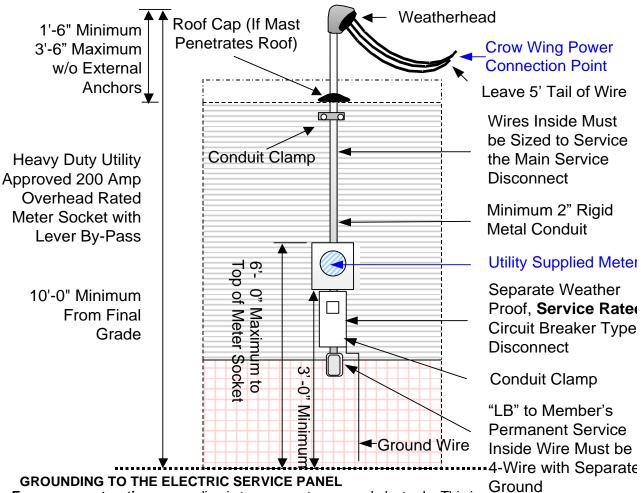
For new construction, grounding is to a concrete encased electrode. This is:
